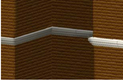
Jamison Midline Banding; Straights, Cope Outside Rights, Cope Outside Lefts, Cope Inside Rights, and Cope Inside Lefts.
