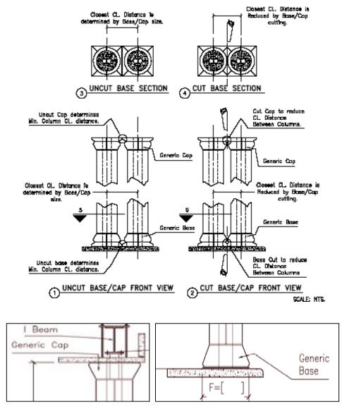
Many columns are designed to be load bearing and support structures above that require both base and cap cutting to fit attachment assemblies or weld plates. See next pages Installation Information for more detailed explanations.
