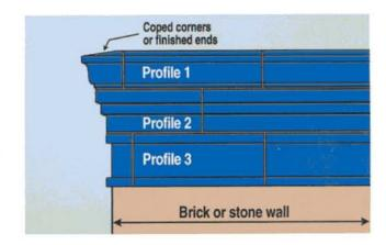
A banded wall or pier cap is made up of profiled stones that are sold by the linear foot, including cast-in corners. They may be a single profile or stacked. Almost any profiles can be used, but they must stack properly atop one another. See Chapter 11 - Profiles: The DNA of Stone for more information on stacking profiles.
