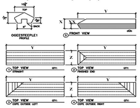
All Pieces are 36 in and can be cut in the field for fitting. Finshed ends, Mitre cutting and Radius options available.
