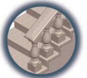
Volute End This Volute Ended handrail, right, has no baserail. Note that the bottom baluster was lengthened to accommodate the difference in height. The rounded bottom step is referred to as a starter step.
