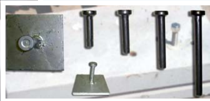
Weld plate imbed and nelson bolts. Used commercially in most cases.
