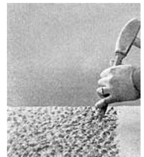
Historically, a point finish was achieved with a pointed chisel. Photo: From the Stone Company Catalog. Courtesy: F. Lynch.
