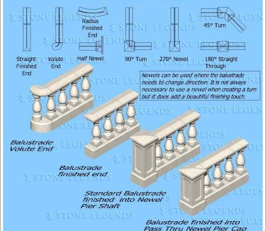
There are various options available to finish balustrade. Examples shown above include a volute end and a finished end. Also shown is where the balustrade terminates into a newel pier. With newel piers there are two key options. The first option is to run the handrail into the newel pier shaft or alternatively into the pier cap.
